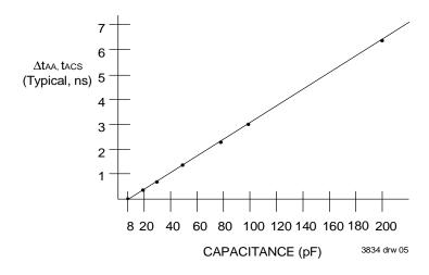
Figure 3. Output Capacitive Derating
