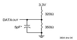
${}^{\star}\text{Including jig and scope capacitance}.$
